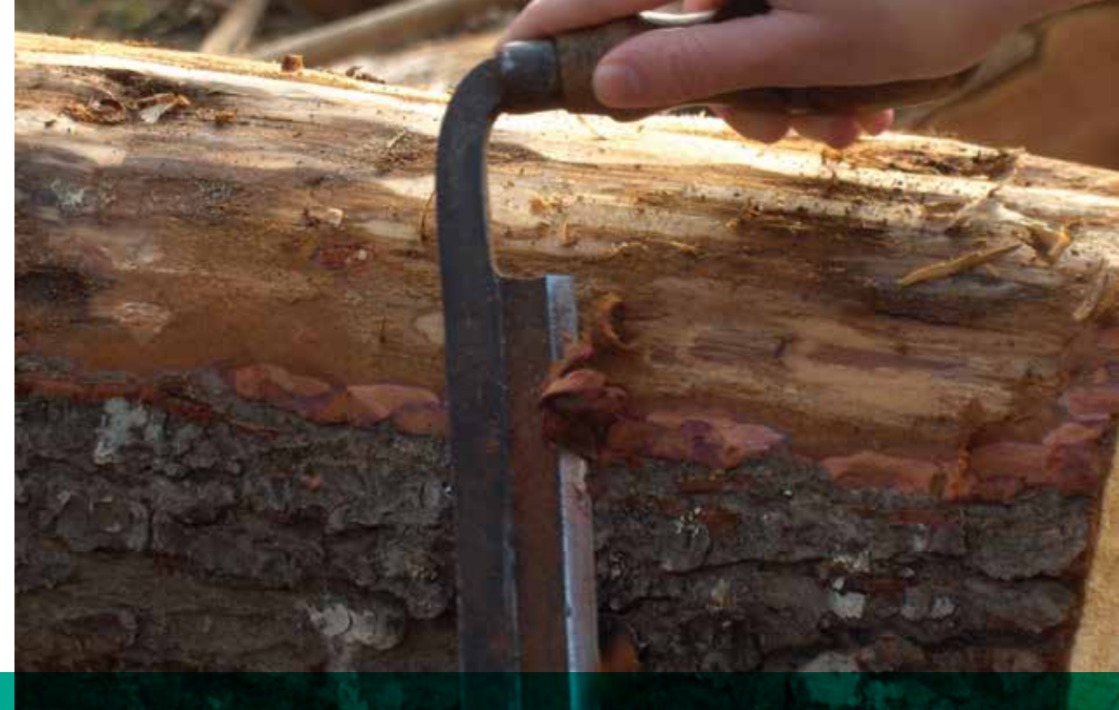
Left: Masonry detail; Center: Comstock Barn at Ebey's Landing National Historical Preserve on Whidbey Island, Washington, Photo: Courtesy of PNWFS. Right: Using a drawknife to prepare a log, Olympic National Park. Photo: Courtesy of PNWFS.
