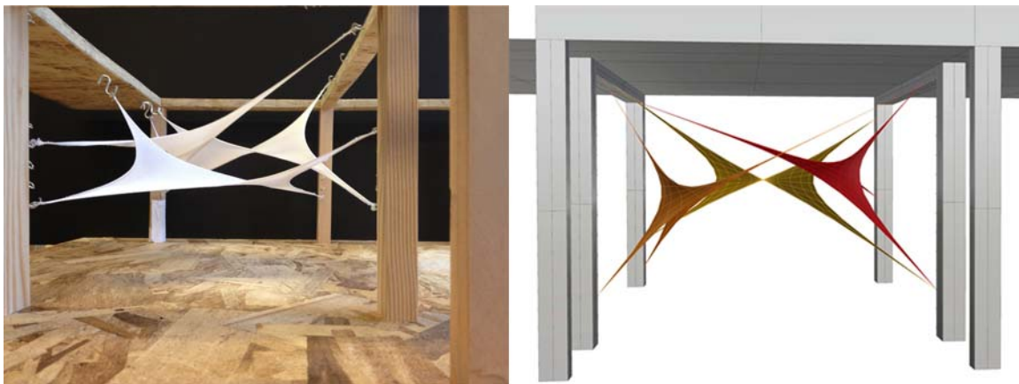
Figure 4: Physical and digital form-finding models utilized to optimize installation configuration and variables.
